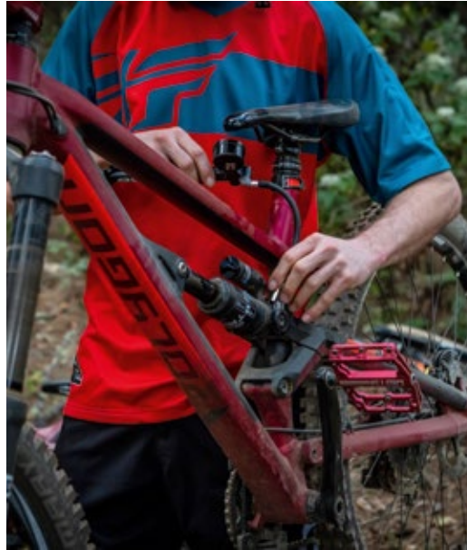
LEFT Kurt and James chasing each other through the winding forests trails kicking up pine needles and fine dust. TOP Kurt makes some quick volume spacing changes to his TRIAir 3CR to make his spring curve more progressive for the steep, rugged trails.
