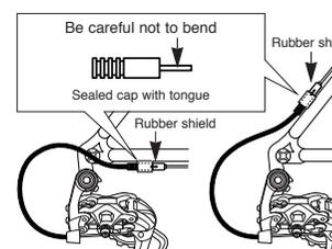
\* If the rear derailleur moves to a large degree, such as in bicycles with rear suspension, it is recommended that you replace the cap with the accessory aluminum cap.
