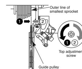
Connect the cable to the rear derailleur and, after taking up the initial slack in the cable, re-secure to the rear derailleur as shown in the illustration.
